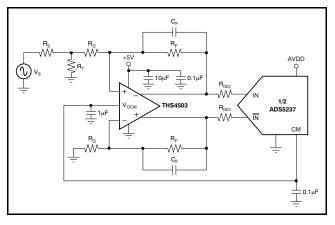
Figure 19. Using the THS4503 with the ADS5237
