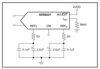
Figure 20. Internal Reference Circuit
