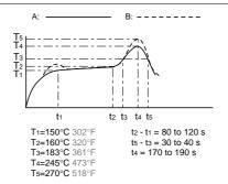
Temperature rise of relay itself may vary according to the mounting level or the heating method of reflow equipment. Therefore, please set the temperature of soldering portion of relay terminal and the top surface of the relay case not to exceed the above mentioned soldering condition. It is recommended to check the temperature rise of each portion under actual mounting condition before use.
