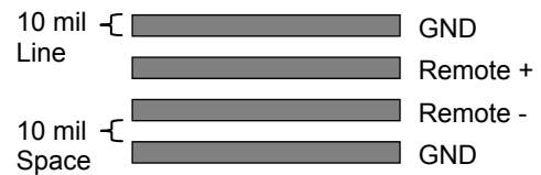
Figure 13 Recommended Remote Diode Circuit Board Interconnect
