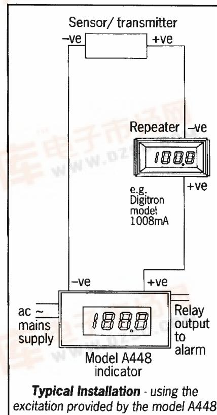
**Typical Installation** - using the excitation provided by the model A448
