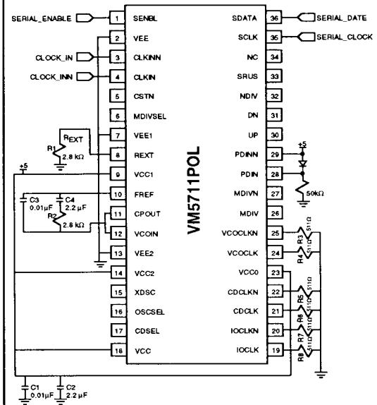
Resistor  $R_{5-17}$  is a  $\pm 1\%$  absolute tolerance in value
