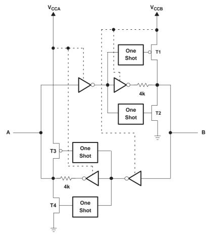
Figure 1. Architecture of TXB0108 I/O Cell
