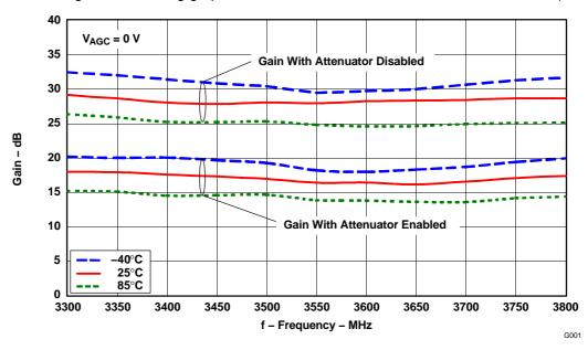
Figure 2. Gain vs Frequency for VAGC = 0 V
