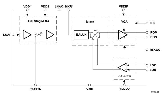
Figure 1. Detailed Block Diagram of TRF1216
