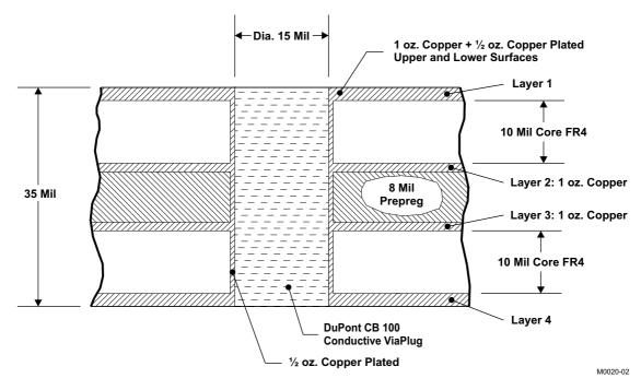
NOTE: Top and bottom surface finish: copper flash with 50–70  $\mu$ in white tin immersion.
