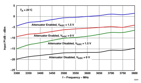
Figure 5. Input P1dB vs Frequency,  $(T_A = 25^{\circ}C)$
