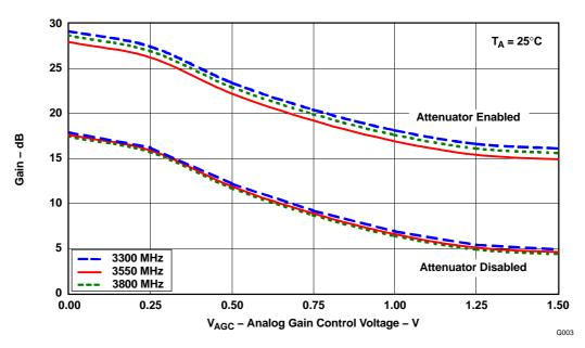
Figure 4. Gain vs VAGC for Different Frequencies,  $(T_A = 25^{\circ}C)$
