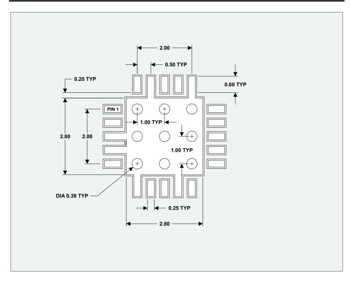
Solder Mask. No Solder Mask Under Chip, On Lead Pads or On Ground Connections.
