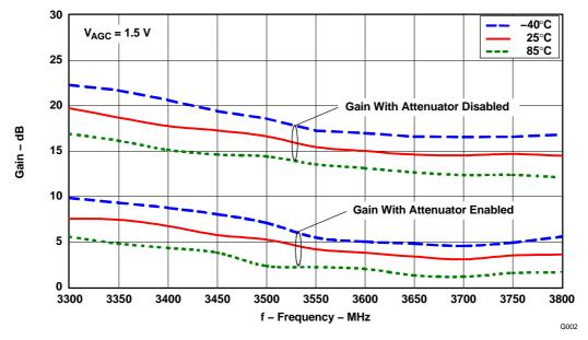
Figure 3. Gain vs Frequency for VAGC = 1.5 V
