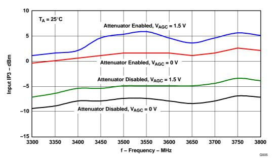
Figure 6. Input IP3 vs Frequency,  $(T_A = 25^{\circ}C)$
