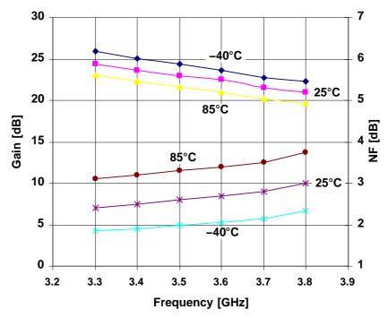
Figure 7. LNA Noise Figure vs Frequency With VAGC = 0 V
