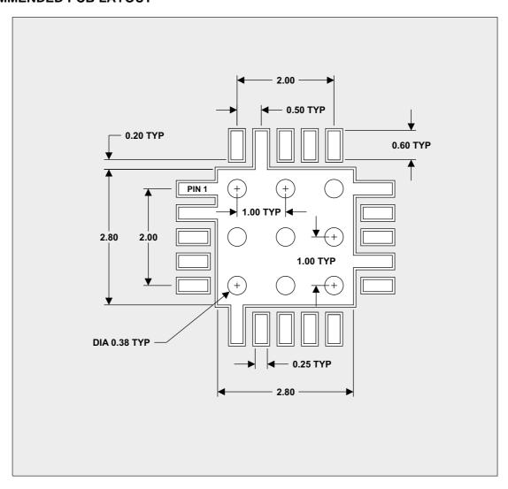
Solder Mask. No Solder Mask Under Chip, On Lead Pads or On Ground Connections.
