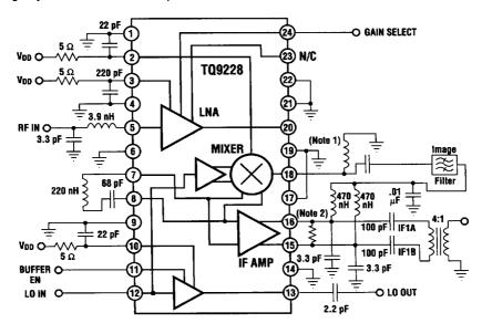
Notes: 1. Optional shunt inductance and series capacitance to improve the input matching. 2. Optional resistor to adjust gain.
