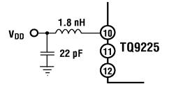
IF  $V_{\text{DD}}$  – The IF outputs are biased through chokes connected to  $V_{\text{DD}}.$  The supply end of the inductors requires a decoupling capacitor.
