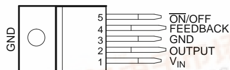
KV (TO-220 STAGGERED LEADS) PACKAGE (TOP VIEW)
