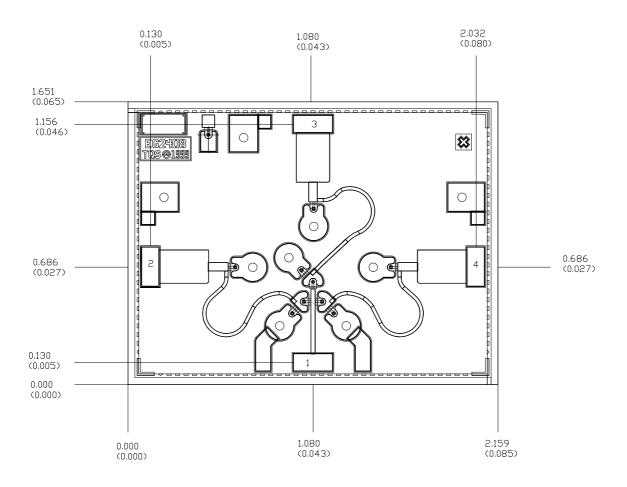
Units: millimeters (inches) Thickness: 0.100 (0.004)
