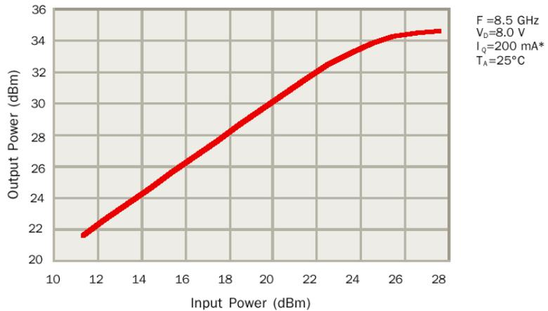
\*  $I_Q$  is defined as the drain current before application of RF signal at the input.
