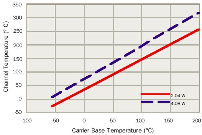
38 μm AuSn solder attach to 0.5 mm CuMo Carrier.
