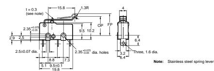
Hinge Lever SS-01GL2(-E, -F) SS-5GL2(-F)
