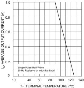
T<sub>T</sub>, TERMINAL TEMPERATURE (°C) Fig. 1 Forward Current Derating Curve
