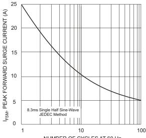
NUMBER OF CYCLES AT 60 Hz Fig. 3 Maximum Non-Repetitive Peak Fwd Surge Current
