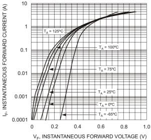
Fig. 2 Typical Forward Characteristics
