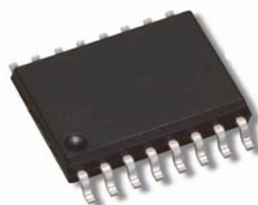
Figure 1 : Image of TSSOP -16 Exposed Paddle Plastic Package
