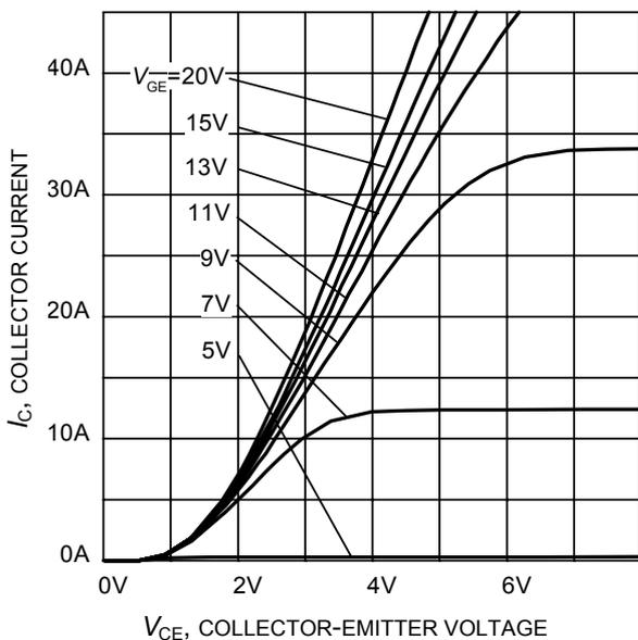
**Figure 5. Typical output characteristic**
