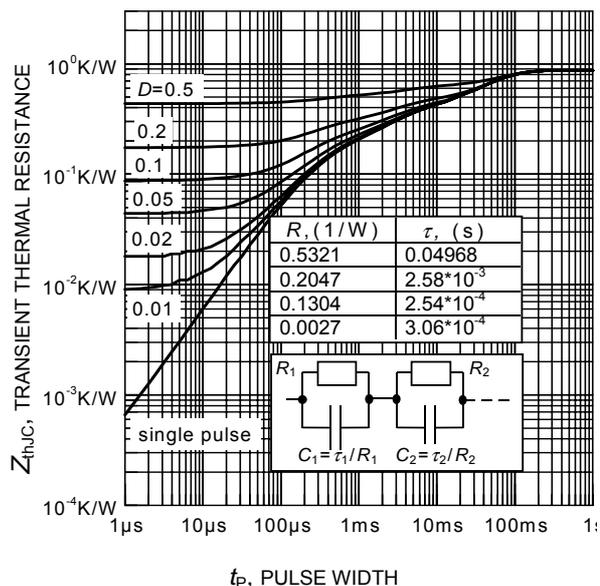
**Figure 16. IGBT transient thermal resistance** ( $D = t_p / T$ )
