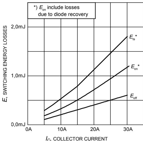
**Figure 13. Typical switching energy losses as a function of collector current** (inductive load,  $T_J=150^\circ\text{C}$ ,  $V_{CE}=400\text{V}$ ,  $V_{GE}=0/15\text{V}$ ,  $R_G=23\Omega$ , Dynamic test circuit in Figure E)
