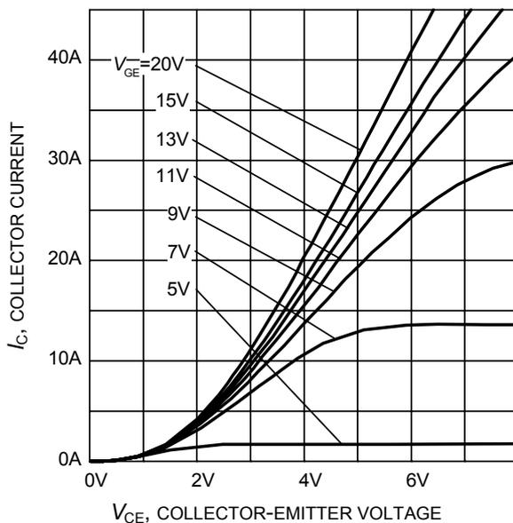
**Figure 6. Typical output characteristic**
