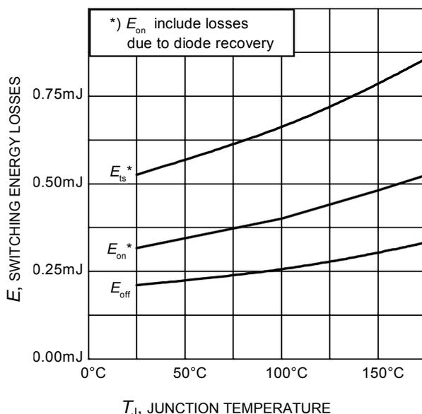
**Figure 15. Typical switching energy losses as a function of junction temperature** (inductive load,  $V_{CE}=400\text{V}$ ,  $V_{GE}=0/15\text{V}$ ,  $I_C=20\text{A}$ ,  $R_G=23\Omega$ , Dynamic test circuit in Figure E)
