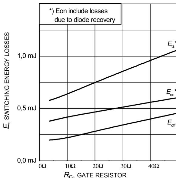
**Figure 14. Typical switching energy losses as a function of gate resistor** (inductive load,  $T_J=150^\circ\text{C}$ ,  $V_{CE}=400\text{V}$ ,  $V_{GE}=0/15\text{V}$ ,  $I_C=15\text{A}$ , Dynamic test circuit in Figure E)
