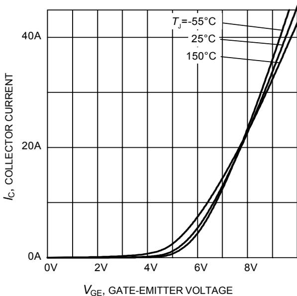
**Figure 7. Typical transfer characteristic**
