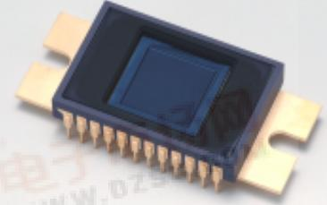
S8844-0909 is an FFT-CCD area image sensor developed for measurement of low-light-level. S8844-0909 has a back-thinned structure for detecting light from the backside that allows high sensitivity from UV to near infrared region. S8844-0909 also delivers a wide dynamic range and low dark current when operated in MPP (Multi Pinned-Phase) mode. Spectral response characteristics are very stable making high-precision photometry possible.
