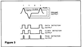
output and shift it in time. The phase-shift capacitor is selected to provide additional phase-shift so that the strobe pulses will occur at the center of the incoming pulses. This provides optimum timing for determining if a "1" or a "0" is present. A 0-to-30pF capacitor (10pF is typical at 1.544MHz) will optimize the performance of the complete repeater.
