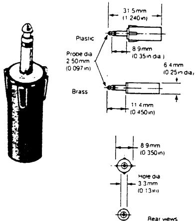
good contact resistance and solderability. Two styles of cover are available black thermoplastic and nickel plated brass. The
