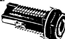
Gold flash spring contacts made from phosphor bronze to give good solderability and corrosion resistance with a nickel plated locating washer used to prevent socket rotation in the panel.
