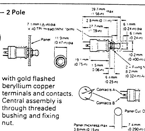
with gold flashed beryllium copper terminals and contacts. Central assembly is through threaded bushing and fixing nut.
