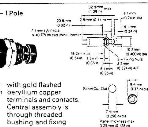
with gold flashed beryllium copper terminals and contacts. Central assembly is through threaded bushing and fixing nut.
