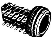
Fixed by a plastic nut with disposable washers provided for panel thickness adjustment. The thread end is hidden by a plastic fixing nut which screws into the socket. Gold flashed spring contacts made from phosphor bronze give good solderability and corrosion resistance. Spring life is enhanced by the generous curve at the fixed ends.
