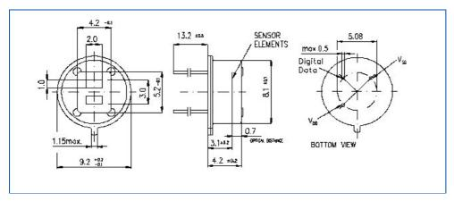
PIN Layout. All measurements are in mm.
