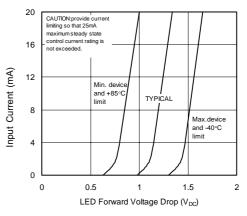
Figure 6. Input Characteristics (Current Controlled)
