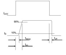
Figure 7. Typical Delay Times
