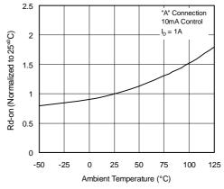
Figure 4. Typical Normalized On-Resistance
