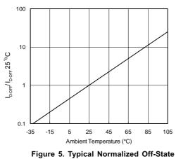
Figure 5. Typical Normalized Off-State Leakage
