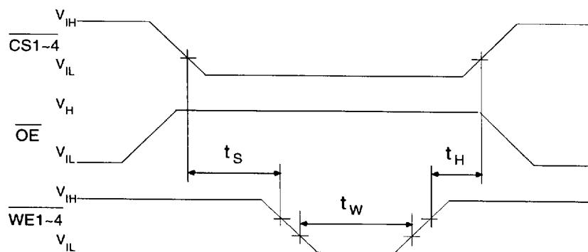
$t_s = t_h = 5\mu s \text{ (min)}$     $t_w = 10 \text{ ms (min)}$     $V_H = 12V \pm 0.5V$
