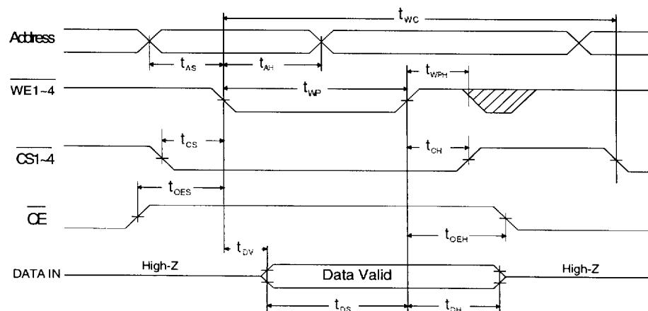
**AC Write Waveform - CS1~4 Controlled**
