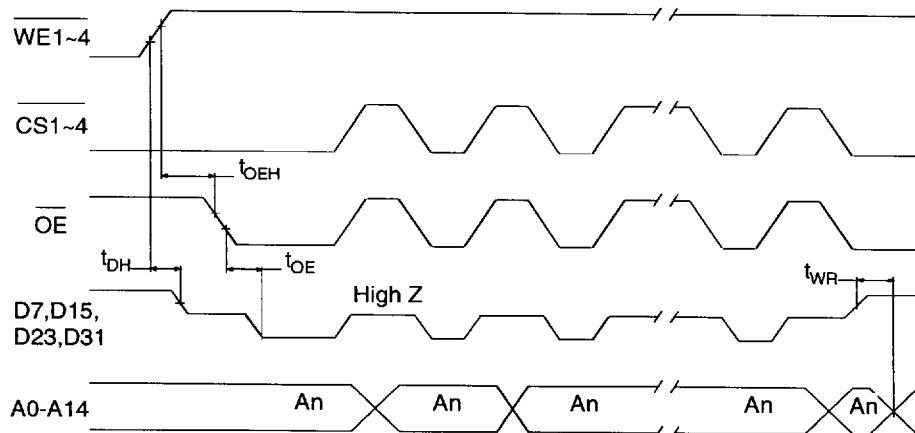
**Toggle Bit Waveform (1,2,3,4)**
