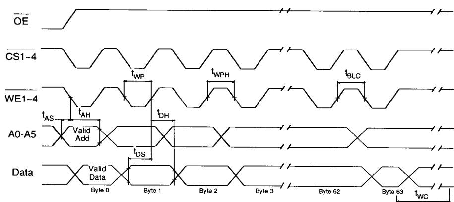
Note: (1) A6 through A14 must specify the page address during each high to low transition of WE1~4 (or CS1~4).
