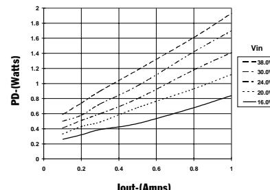
**Note 1:** All data listed in the above graphs, except for derating data, has been developed from actual products tested at 25°C. This data is considered typical data for the ISR.
