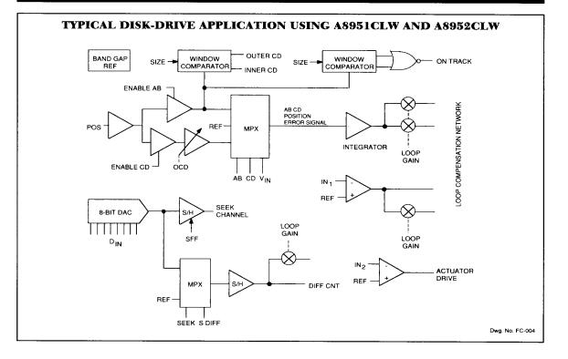
Voice-coil servo motors in disk-drive head-positioning systems utilize complex algorithms and sophisticated circuitry to provide good track-seeking and track-following performance. A typical hard-disk track geometry requires precise voice-coil motor control to ensure accurate positioning of the head above the desired track.
