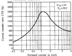
Fig. 7 Relative Current Transfer Ratio vs.
