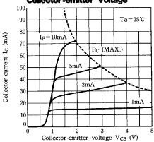
Fig. 8 Collector-emitter Saturation Voltage
