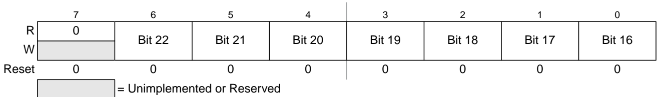
Figure 20-15. Debug Comparator Address High Register (DBGXAH)
