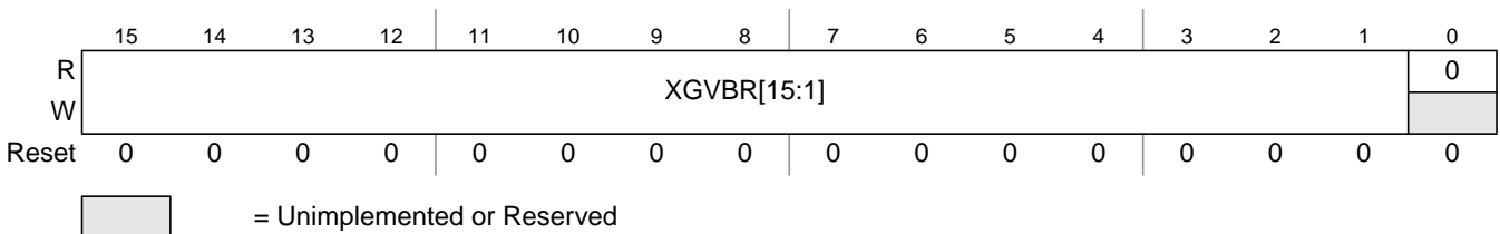
Figure 6-5. XGATE Vector Base Address Register (XGVBR)
