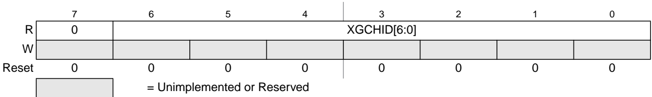
Figure 6-4. XGATE Channel ID Register (XGCHID)
