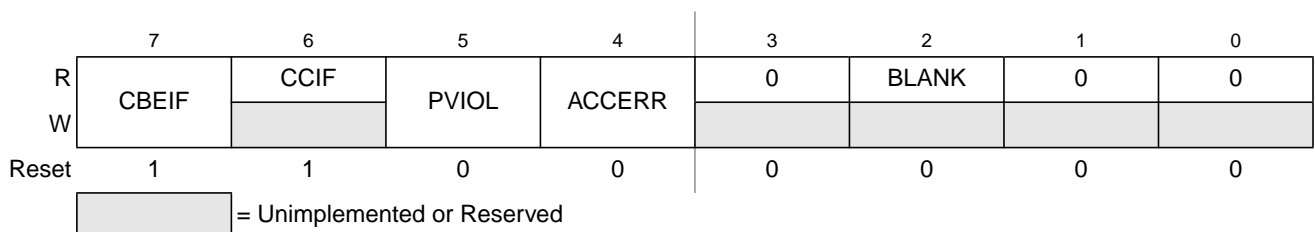
Figure 28-12. Flash Status Register (FSTAT — Normal Mode)
