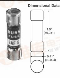
CATALOG SYMBOL: BAF (5AG) **FAST-ACTING** 2/10 TO 30 AMPERES U.L. RECOGNIZED, STD. 248-14 0-15/250V AC (GUIDE # JDYX, FILE # E19180) **CSA CERTIFIED**
