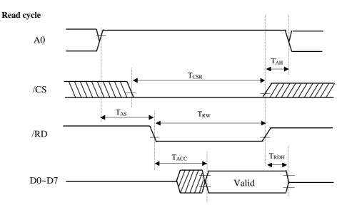
Note:  $T_{ACC}$  is defined with respect to the moment /CS or /RD becomes Low level later.
