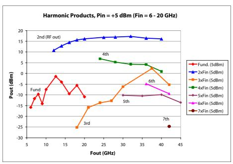
\* Measured on-wafer with die version of doubler.
