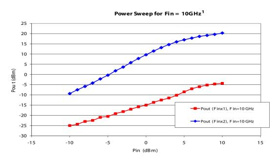
1. Measured results taken at room temperature in 40 GHz connectorized test fixture with no de-embedding.
