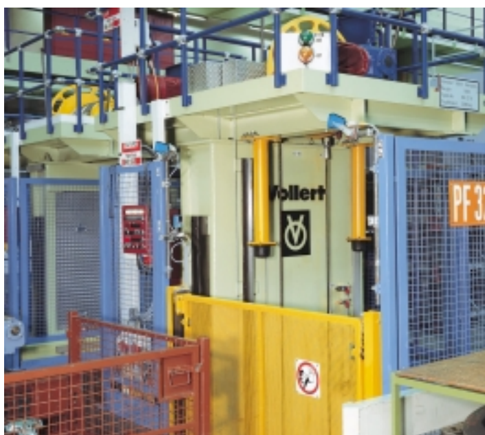
▲ WL 36 sensors used to detect mesh baskets in front of a goods lift.
