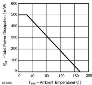
Fig. 1 Total Power Dissipation vs. Ambient Temperature
