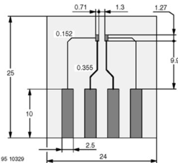
Fig. 10 Board for  $R_{thJA}$  definition (in mm)
