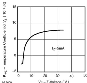
Fig. 3 Temperature Coefficient of V<sub>Z</sub> vs. Z-Voltage
