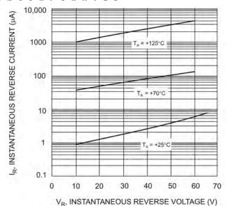
Fig. 7 Typical Reverse Characteristics, B350B thru B360B
