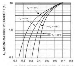
$V_{\rm F}$ , INSTANTANEOUS FORWARD VOLTAGE (V) Fig. 2 Typical Forward Characteristics - B320B thru B340B
