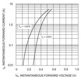
Fig. 3 Typ. Forward Characteristics - B350B thru B360B
