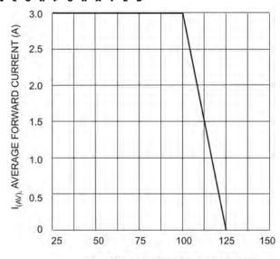
T<sub>T</sub>, TERMINAL TEMPERATURE (°C) Fig. 1 Forward Current Derating Curve
