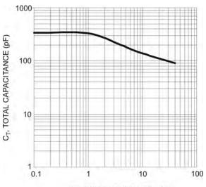
V<sub>R</sub>, REVERSE VOLTAGE (V) Fig. 5 Typical Capacitance
