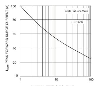
NUMBER OF CYCLES AT 60 Hz Fig. 4 Max Non-Repetitive Peak Forward Surge Current
