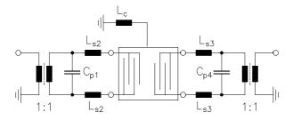
$$\begin{array}{lll} L_c & = 39 \text{ nH} \\ C_{p1} & = C_{p4} = 6.8 \text{ pF} \\ L_{s2} & = L_{s3} = 33 \text{ nH} \end{array}$$
