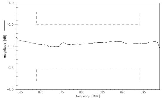
Output phase balance ( $\phi(S_{31})-\phi(S_{21})+180^{\circ};$  50  $\Omega$  to 150  $\Omega$  operation)
