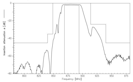
Transfer function (wideband; 50  $\Omega$  to 150  $\Omega$  operation)
