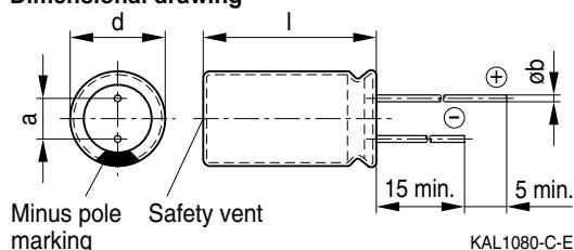
Safety vent for diameter  $\geq 8$  mm.
