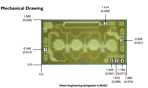
Units: millimeters (inches) Bond pad dimensions are shown to center of bond pad. Thickness: 0.076 + /- 0.010 (0.003 + /- 0.0004), Backside is ground, Bond Pad/Backside Metallization: Gold All DC Bond Pads are  $0.080 \times 0.080 (0.003 \times 0.003)$ . All RF Bond Pads are  $0.180 \times 0.080 (0.007 \times 0.003)$ . Bond pad centers are approximately 0.109 (0.004) from the edge of the chip.
