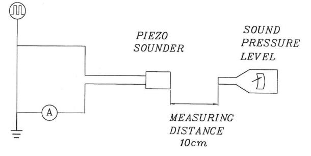
S.P.L. Measuring Circuit Input Signal: 5 V p-p, 4.1 KHz, Square Wave Mic: RION UC 30 S.G.: Hewlett Packard 33120A Function Generator or equivalent
