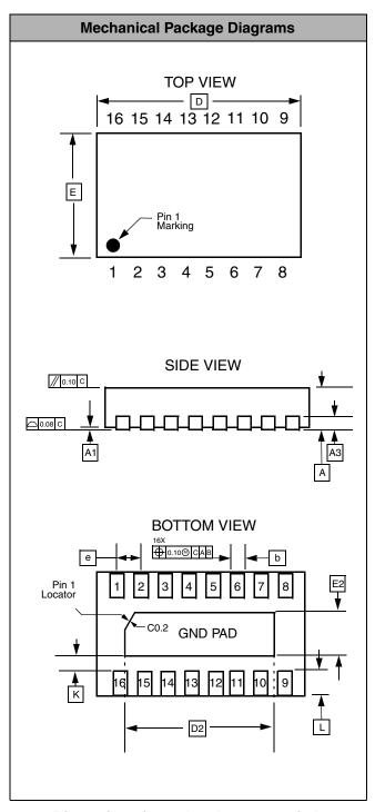
Dimensions for 16-Lead, 0.75mm pitch TDFN package
