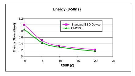
Figure 5. Energy Dissipated in DUP vs RDUP\*
