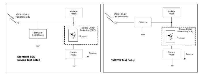
Figure 6. Test Setups: Standard Device (Left) and CM1233 (Right)
