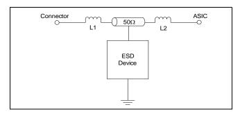
Figure 3. CM1233 *PicoGuard XS* ESD Protection Model
