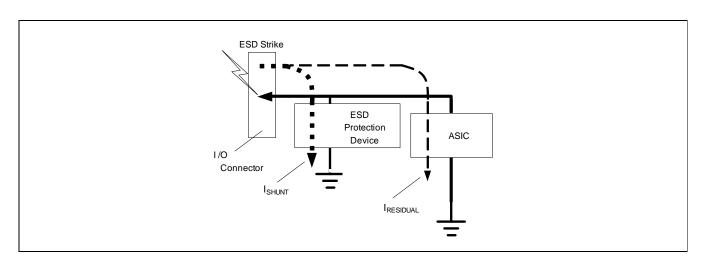
Figure 1. Standard ESD Protection Device Block Diagram
