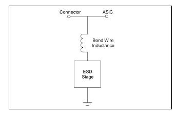
Figure 2. Standard ESD Protection Model
