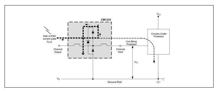
Figure 8. Application of Positive ESD Pulse Between Input Channel and Ground
