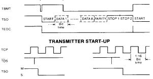
Upon da:a transmission initiation, or when not transmitting at 100% line utilitzation, the start bit will be placed on the TSO line at the high to low transition of the TCP clock following the trailing edge of  $\overline{\text{TDS}}$ .
