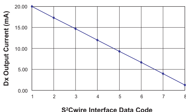
Figure 3: AAT3192-2 Current Control Profile.
