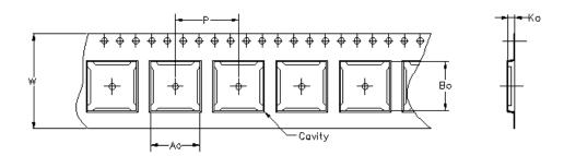
Carrier tape design is defined largely by the component lentgh, width, and thickness.
