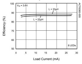
Efficiency vs. Load Current
