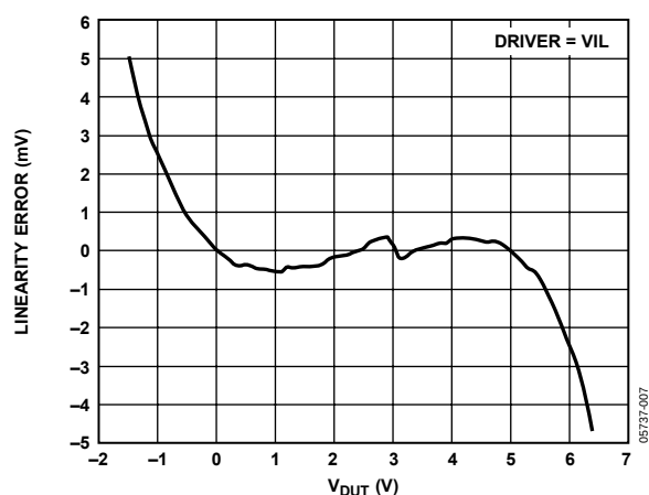
Figure 7. Driver VIL Linearity vs. Output
