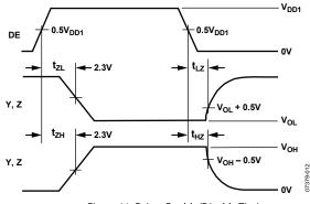
Figure 11. Driver Enable/Disable Timing
