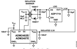
Figure 34. Applications Diagram
