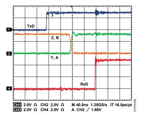
Figure 29. ADM2482E Driver/Receiver Propagation Delay, Low to High  $(R_{DIFF}=54~\Omega,~C_{L1}=C_{L2}=100~pF)$
