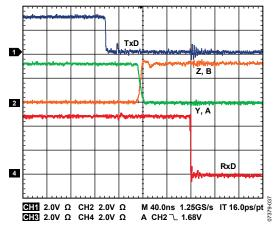
Figure 28. ADM2482E Driver/Receiver Propagation Delay, High to Low  $(R_{DIFF}=54~\Omega,~C_{L1}=C_{L2}=100~pF)$
