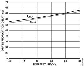
Figure 19. ADM2482E Driver Propagation Delay vs. Temperature
