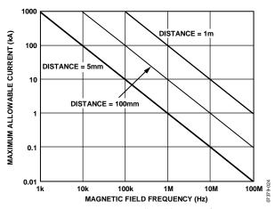
Figure 32. Maximum Allowable Current for Various Current-to-ADM2482E/ADM2487E Spacings
