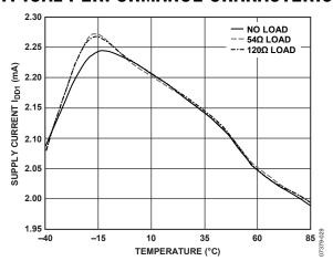
Figure 14. ADM2487E  $I_{DD1}$  Supply Current vs. Temperature (Data Rate = 500 kbps,  $V_{DD1}$  = 5 V,  $V_{DD2}$  = 3.3 V, DE = 1 V,  $\overline{RE}$  = 0 V)
