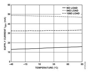
Figure 17. ADM2482E Supply Current vs. Temperature (See Figure 8) (Data Rate = 16 Mbps,  $V_{DD1}$  = 5 V,  $V_{DD2}$  = 3.3 V, DE = 1,  $\overline{RE}$  =0 V)
