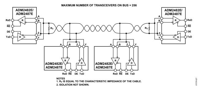
Figure 35. ADM2482E/ADM2487E Typical Half-Duplex RS-485 Network
