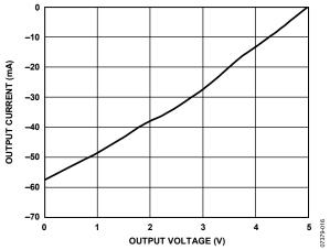
Figure 20. Output Current vs. Receiver Output High Voltage
