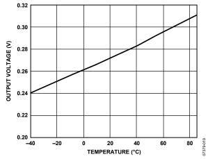
Figure 23. Receiver Output Low Voltage vs. Temperature  $(I_{DD2} = 4 \text{ mA})$
