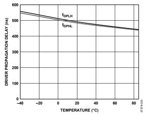
Figure 18. ADM2487E Driver Propagation Delay vs. Temperature
