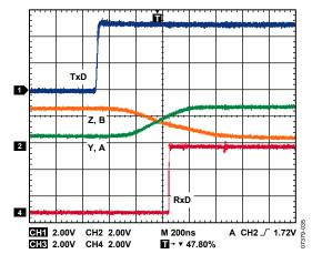
Figure 26. ADM2487E Driver/Receiver Propagation Delay, Low to High  $(R_{DIFF}=54\,\Omega,\,C_{L1}=C_{L2}=100\,pF)$
