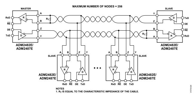
Figure 36. ADM2482E/ADM2487E Typical Full-Duplex RS-485 Network
