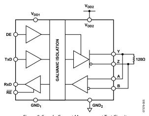
${\it Figure~8. Supply-Current~Measurement~Test~Circuit}$
