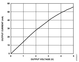
Figure 21. Output Current vs. Receiver Output Low Voltage
