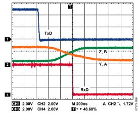
Figure 27. ADM2487E Driver/Receiver Propagation Delay, High to Low  $(R_{DIFF}=54\,\Omega,\,C_{L1}=C_{L2}=100\,pF)$
