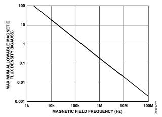
Figure 31. Maximum Allowable External Magnetic Flux Density
