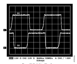
Figure 24. Switching Waveforms (50  $\Omega$  Pull-Up to V<sub>DD1</sub> on D1 and D2)
