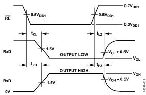
Figure 12. Receiver Enable/Disable Timing
