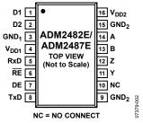
Figure 13. Pin Configuration
