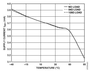
Figure 16. ADM2482E  $I_{DD1}$  Supply Current vs. Temperature (Data Rate = 16 Mbps,  $V_{DD1} = 5 V$ ,  $V_{DD2} = 3.3 V$ , DE = 1 V,  $\overline{RE} = 0 V$ )
