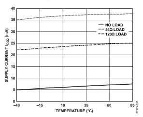
Figure 15. ADM2487E  $I_{DD2}$  Supply Current vs. Temperature (See Figure 8) (Data Rate = 500 kbps,  $V_{DD1}$  = 5 V,  $V_{DD2}$  = 3.3 V, DE = 1 V,  $\overline{RE}$  = 0 V)
