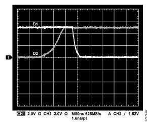
Figure 25. Switching Waveforms (Break-Before-Make,  $50\,\Omega$  Pull-Up to  $V_{DD1}$  on D1 and D2)
