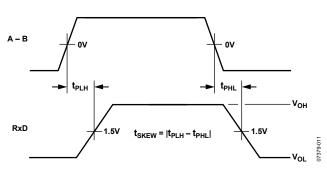
Figure 10. Receiver Propagation Delay
