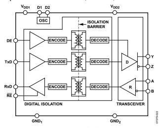
Figure 30. ADM2482E/ADM2487E Digital Isolation and Transceiver Sections
