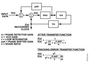
Figure 11. ADN2805 PLL/DLL Architecture
