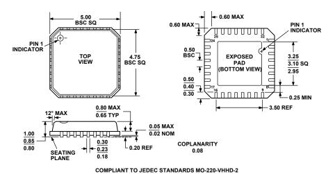
Figure 17. 32-Lead Lead Frame Chip Scale Package [LFCSP\_VQ] 5 mm × 5 mm Body, Very Thin Quad (CP-32-2)
