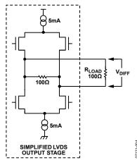
Figure 4. Differential Output Stage
