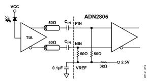
Figure 15. AC-Coupled Input Configuration
