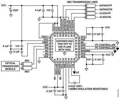
Figure 14. Typical Applications Circuit
