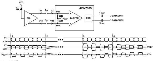
V<sub>DIFF</sub> = V2 – V2b VTH = ADN2805 QUANTIZER THRESHOLD
