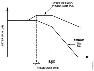
Figure 12. ADN2805 Jitter Response vs. Conventional PLL
