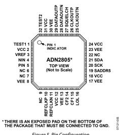
Figure 5. Pin Configuration
