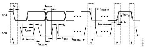
Figure 10.  $I^2C$  Port Timing Diagram
