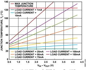
Figure 42. WLCSP, 0 mm<sup>2</sup> of PCB Copper,  $T_A = 25^{\circ}C$
