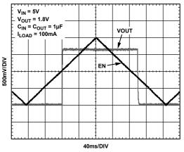
Figure 31. ADP121 Typical EN Pin Operation
