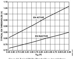
Figure 32. Typical EN Pin Thresholds vs. Input Voltage
