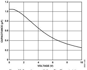
Figure 30. Capacitance vs. Voltage Bias Characteristic
