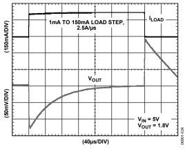
Figure 23. Load Transient Response,  $C_{IN} = C_{OUT} = 1 \ \mu F$
