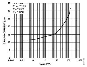
Figure 9. Ground Current vs. Load Current
