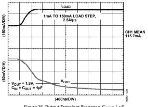
Figure 28. Output Transient Response,  $C_{OUT} = 1 \ \mu F$
