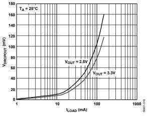
Figure 12. Dropout Voltage vs. Load Current, TSOT
