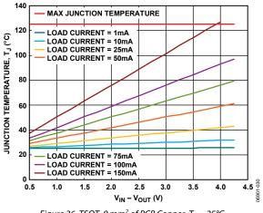
Figure 36. TSOT, 0 mm<sup>2</sup> of PCB Copper,  $T_A = 25^{\circ}C$
