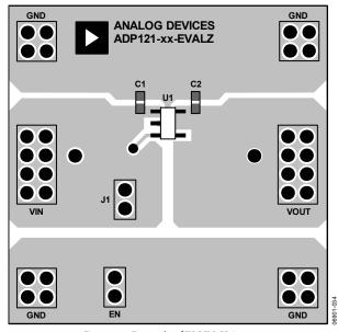
Figure 48. Example of TSOT PCB Layout
