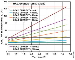
Figure 41. WLCSP, 100 mm<sup>2</sup> of PCB Copper,  $T_A = 25^{\circ}C$
