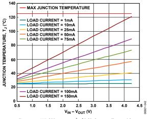
Figure 40. WLCSP, 500 mm<sup>2</sup> of PCB Copper,  $T_A = 25^{\circ}C$
