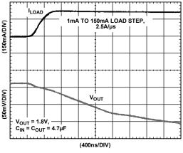
Figure 29. Output Transient Response,  $C_{OUT} = 4.7 \, \mu F$
