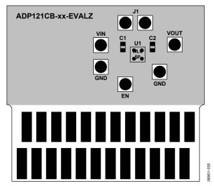
Figure 49. Example of WLCSP PCB Layout
