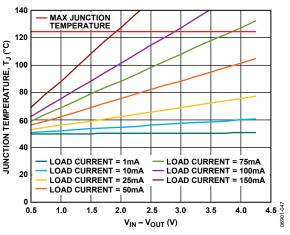
Figure 45. WLCSP, 0 mm<sup>2</sup> of PCB Copper,  $T_A = 50^{\circ}$ C
