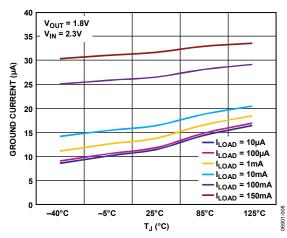
Figure 8. Ground Current vs. Junction Temperature
