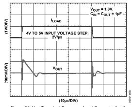
Figure 26. Line Transient Response, Load Current = 1 mA
