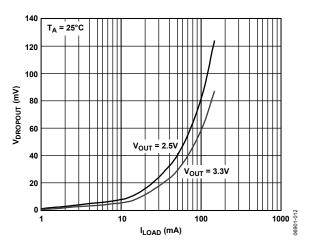
Figure 14. Dropout Voltage vs. Load Current, WLCSP
