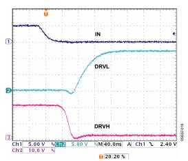
Figure 6. DRVH Fall and DRVL Rise Times  $C_{LOAD} = 6$  nF for DRVH,  $C_{LOAD} = 2$  nF for DRVH
