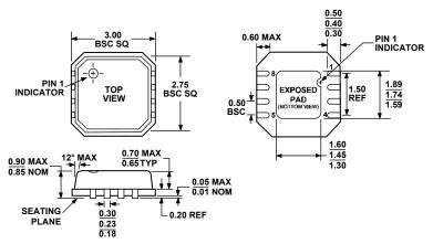
Figure 17. 8-Lead Lead Frame Chip Scale Package [LFCSP\_VD} 3 mm × 3 mm Body, Very Thin, Dual Lead (CP-8-2) Dimensions shown in millimeters
