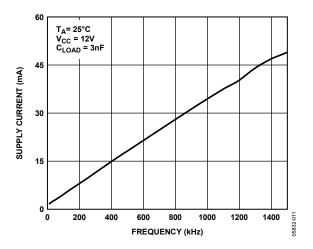
Figure 11. Supply Current vs. Frequency
