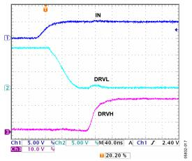
Figure 5. DRVH Rise and DRVL Fall Times  $C_{LOAD} = 6$  nF for DRVH,  $C_{LOAD} = 2$  nF for DRVH
