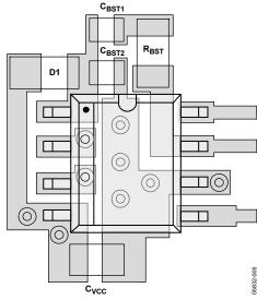
Figure 14. External Component Placement Example
