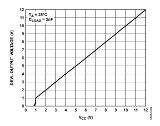
Figure 13. DRVL Output Voltage vs. Supply Voltage
