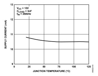
Figure 12. Supply Current vs. Temperature
