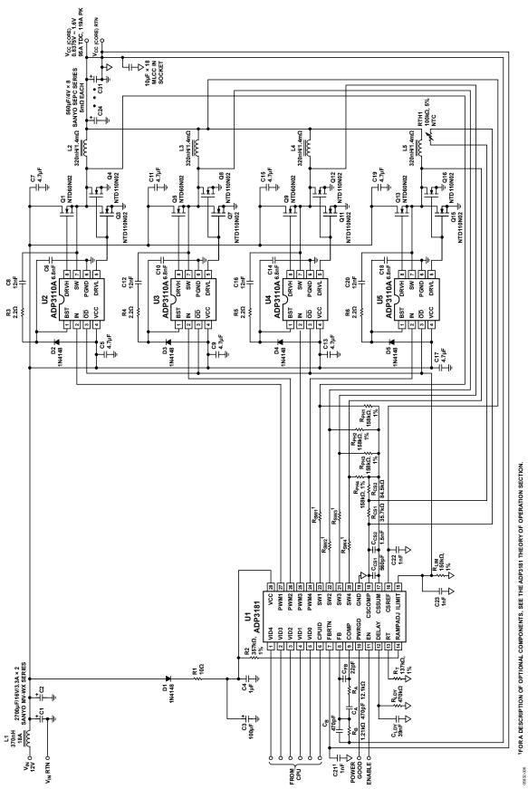
Figure 15. VRD 10.x Compliant Power Supply Circuit
