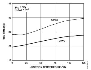
Figure 7. DRVH and DRVL Rise Times vs. Temperature
