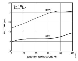
Figure 8. DRVH and DRVL Fall Times vs. Temperature
