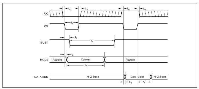
FIGURE 4. Using  $\overline{\text{CS}}$  to Control Conversion and Read Timing.
