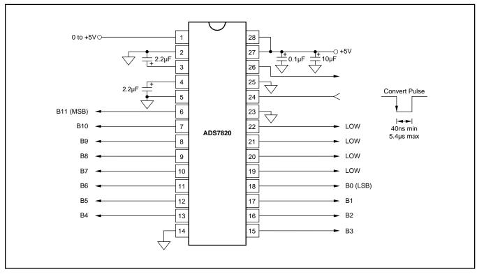
FIGURE 1. Basic Operation (Byte Low).
