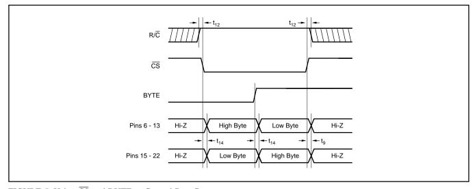
FIGURE 5. Using  $\overline{\text{CS}}$  and BYTE to Control Data Bus.
