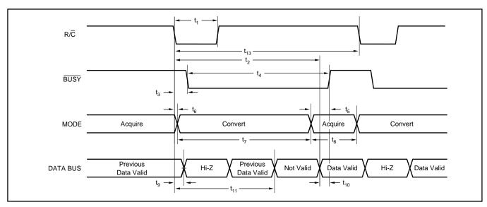
FIGURE 3. Conversion Timing with Outputs Enabled after Conversion ( $\overline{\text{CS}}$  Tied LOW.)
