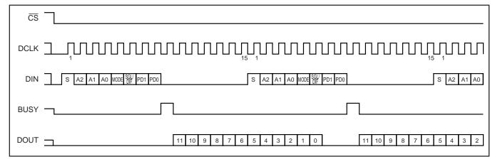
FIGURE 6. Maximum Conversion Rate, 15-Clocks per Conversion.
