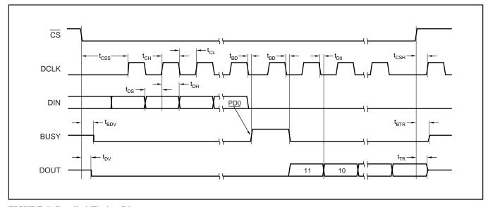
FIGURE 5. Detailed Timing Diagram.
