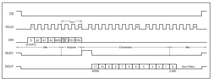
FIGURE 3. Conversion Timing, 24-Clocks per Conversion, 8-Bit Bus Interface. No DCLK delay required with dedicated serial port.
