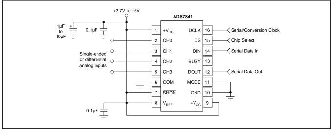
FIGURE 1. Basic Operation of the ADS7841
