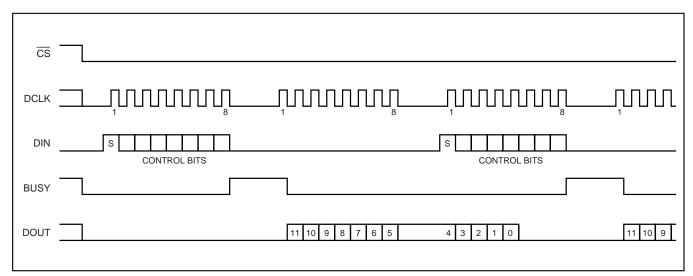
FIGURE 4. Conversion Timing, 16-Clocks per Conversion, 8-bit Bus Interface. No DCLK delay required with dedicated serial port.
